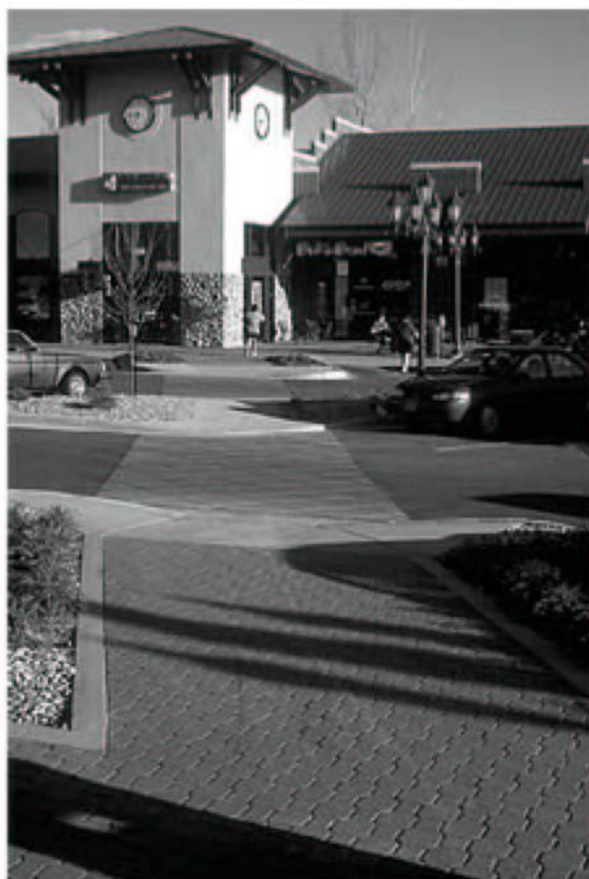
use of special paving where walkways cross a drive aisle or parking area
