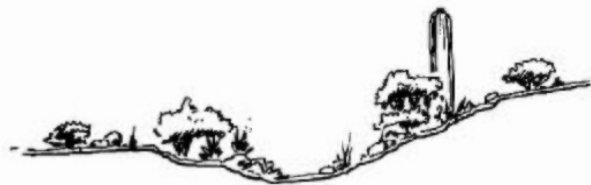
example showing an enhanced natural drainageway as part of the development's stormwater drainage system
