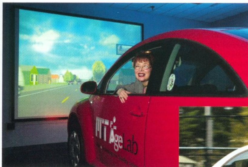
Miss Daisy, a Driving Simulator developed by MIT's AgeLab and the New England University Transportation Center, is used to understand how older drivers use new technology for safe driving. Miss Rosie (below) is an on-road experimental vehicle that assesses driver strength and flexibility.
