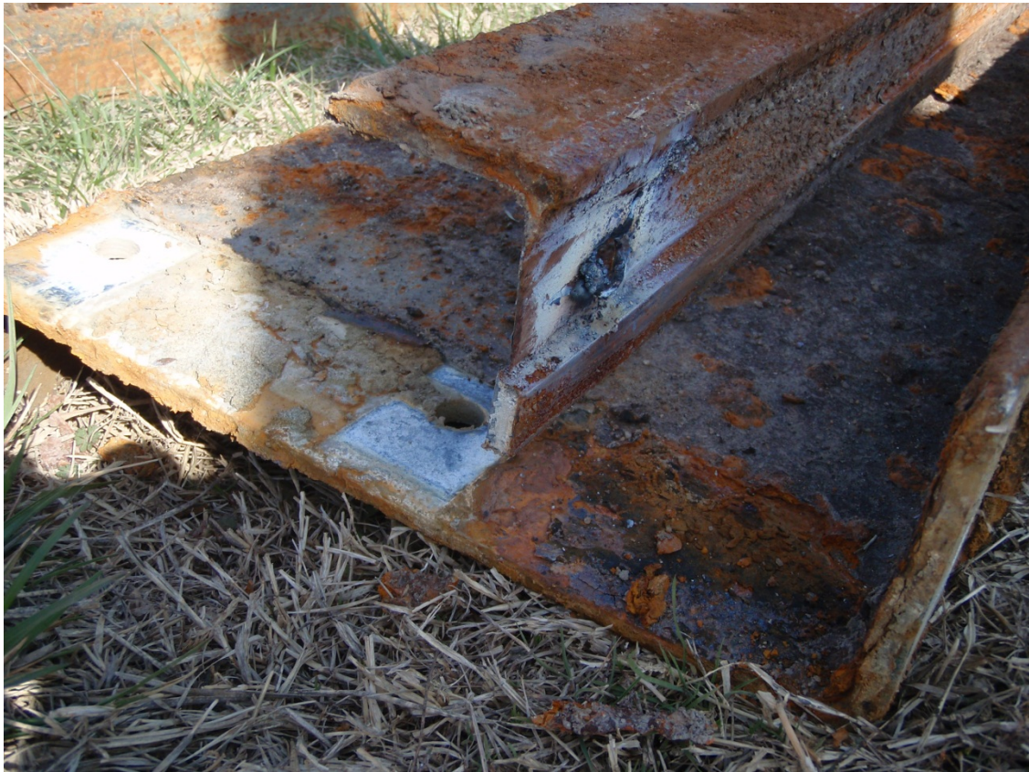
Corroded and worn intermediate frame rail and chain guide
