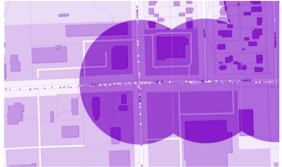
Figure 37: Buffer Area and Crash Spot Locations at W 23rd St & Louisiana
