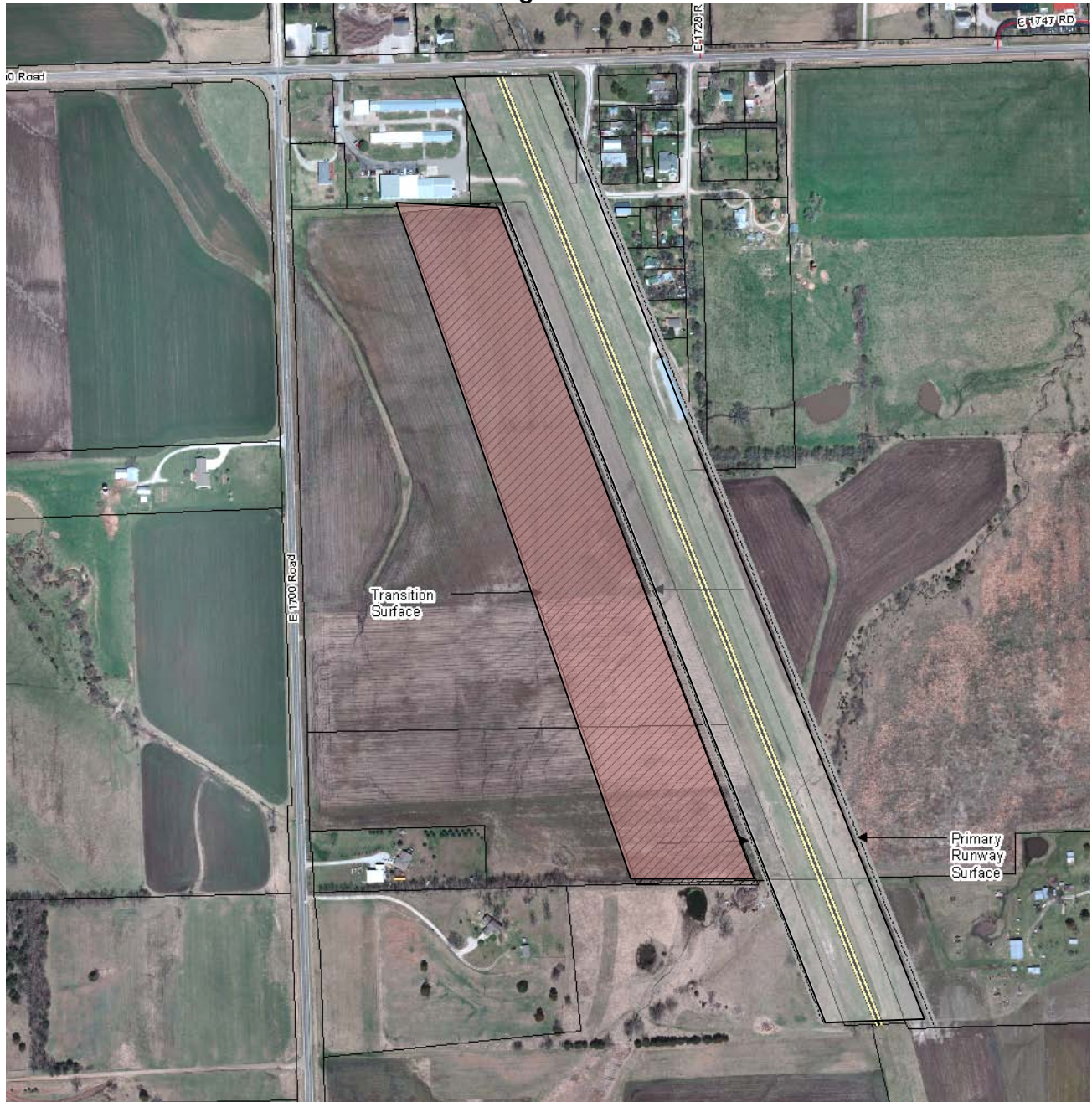
Primary Runway Surface And Transitional Surface Figure 2
